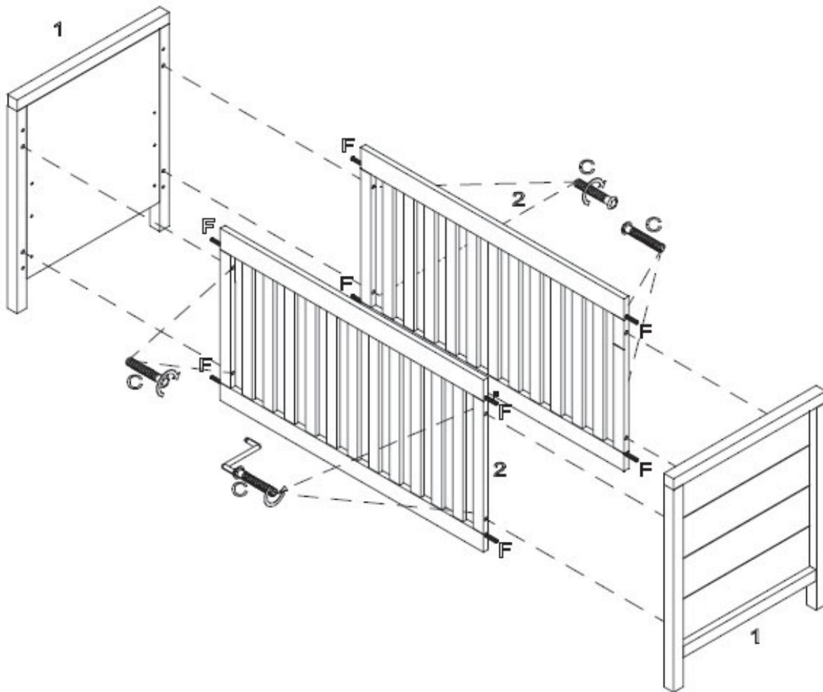
**Step 1** Use the legs **1**, both sides **2**, eight wooden dowels **F**, eight connectors **C** and the hexagonal key **Z**
