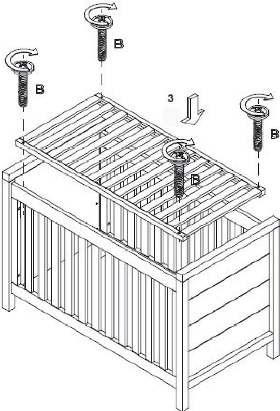
**Step 3 : Use the parts of step 2, the bottom 3 and four wood screws B**
