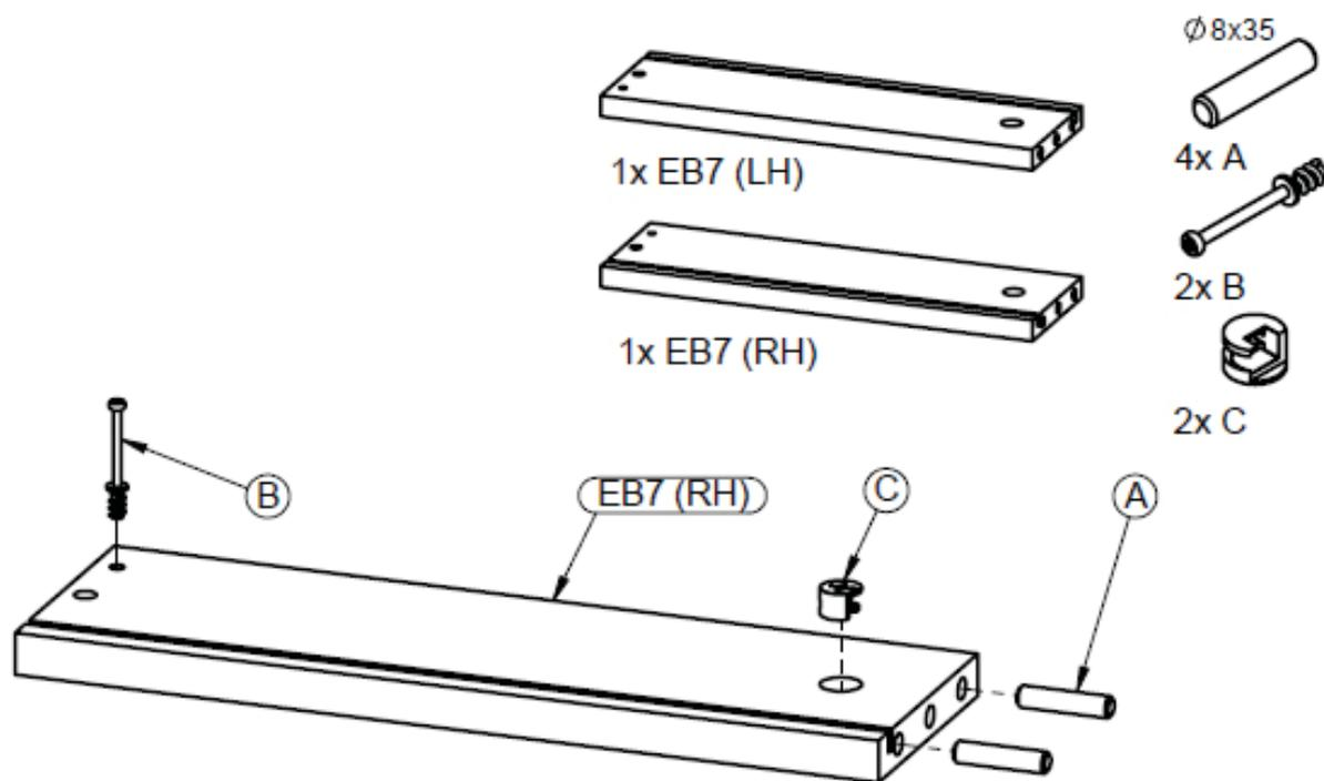
**Step 11 :** Use the left drawer side **EB7 LH** and the right one **EB7 RH**, four wooden dowels **A**, two connectors **B** and two eccentrics **C**
