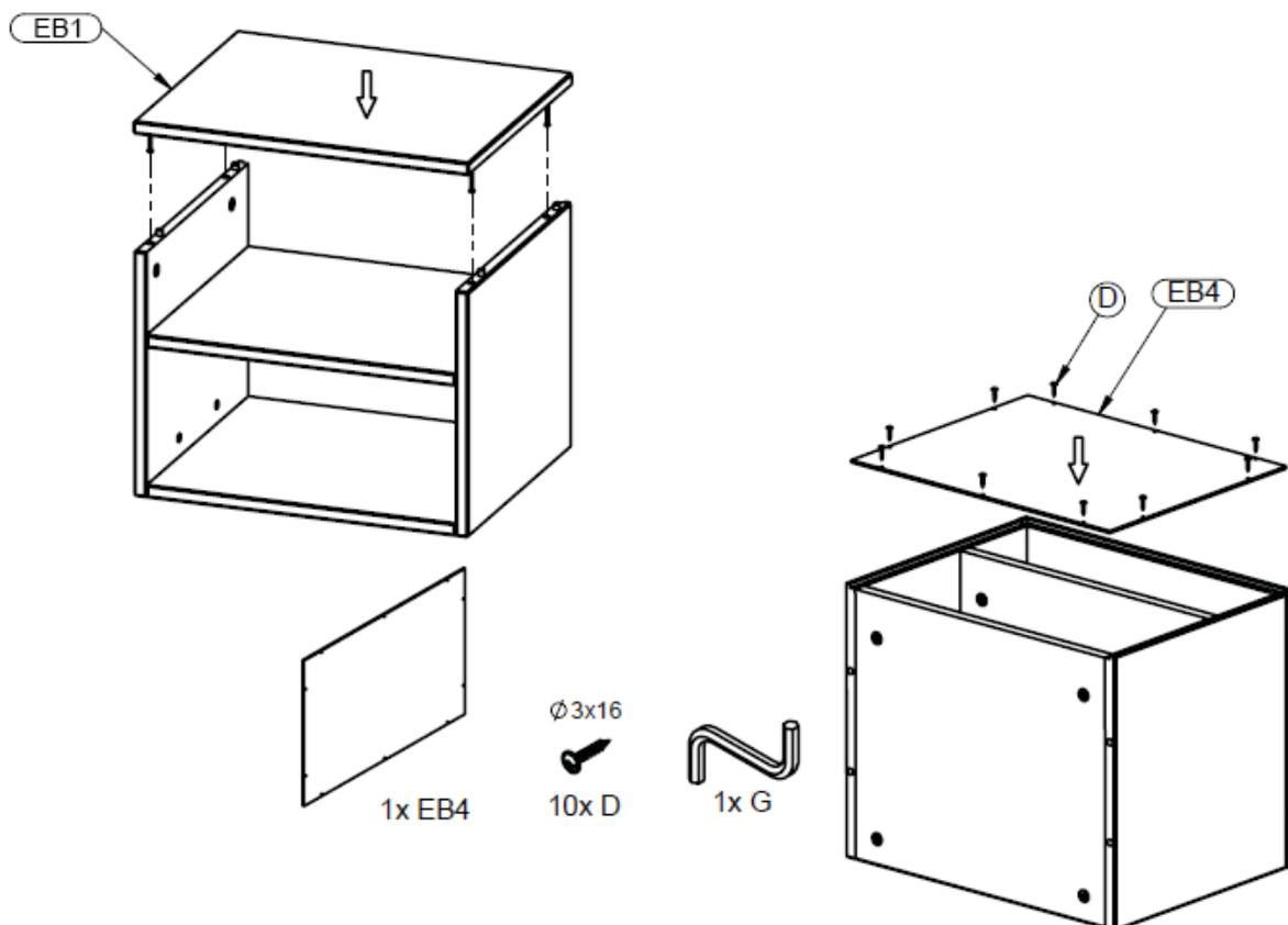
**Step 7 :** Use the parts of step 3 and 6, the back EB4 and ten wood screws D
