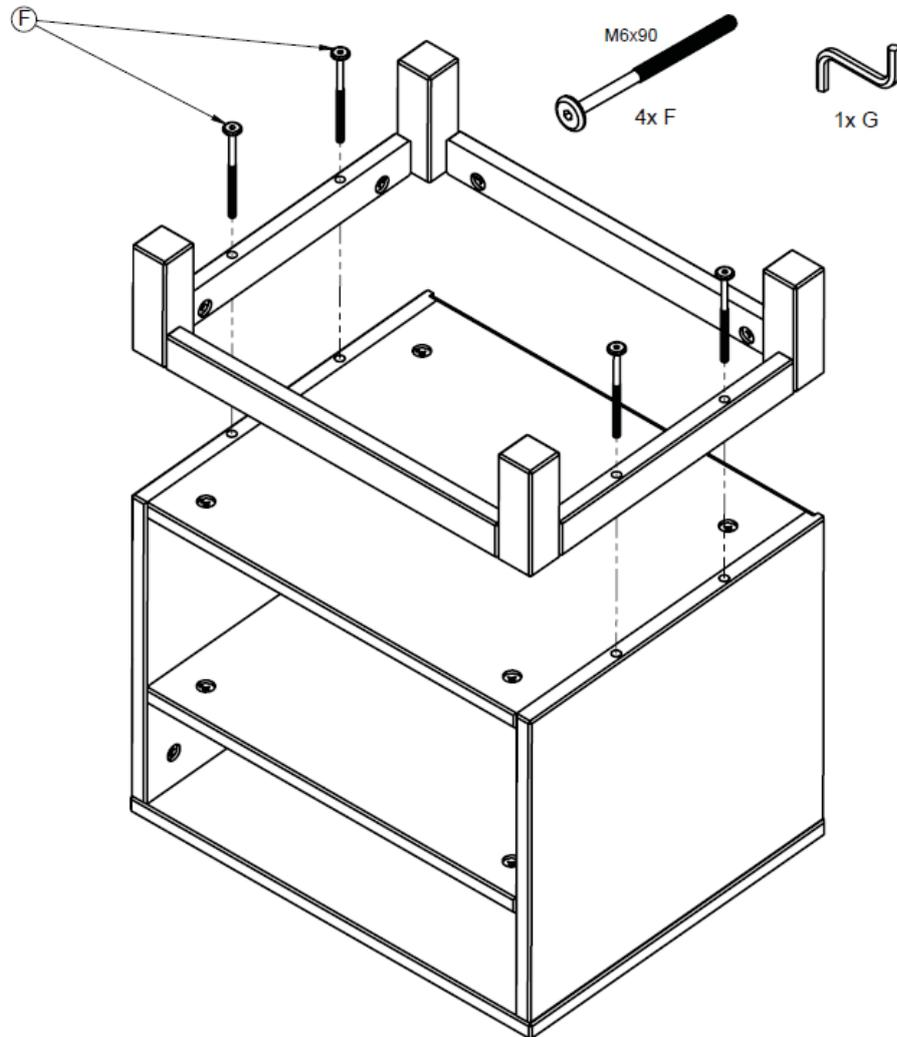
**Step 8 :** Use the parts of steps 2 and 7 and four wood screws **F**
