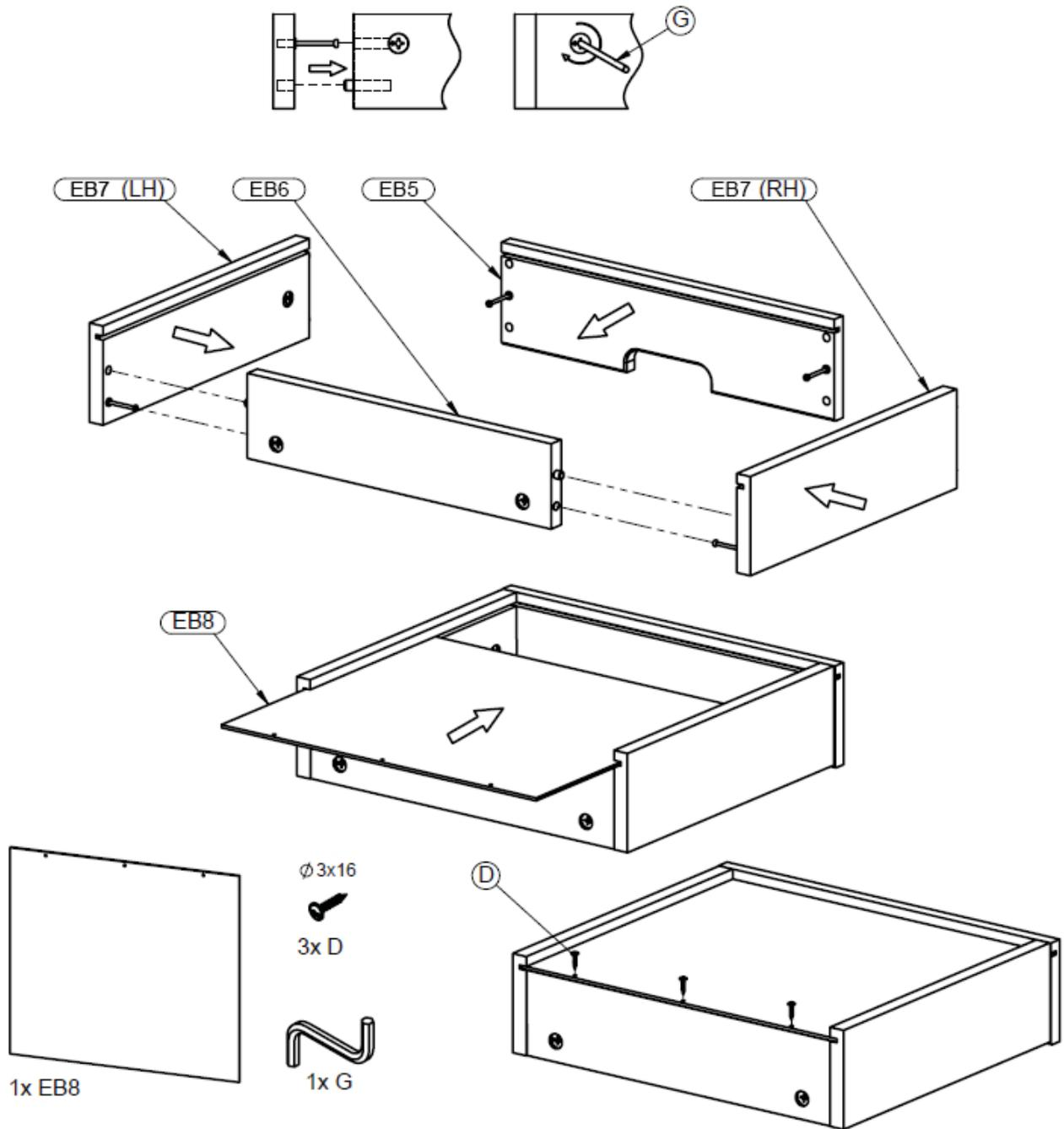
**Step 12 :** Use the parts of steps 9 to 11, the drawer bottom **EB8** and three wood screws **D**
