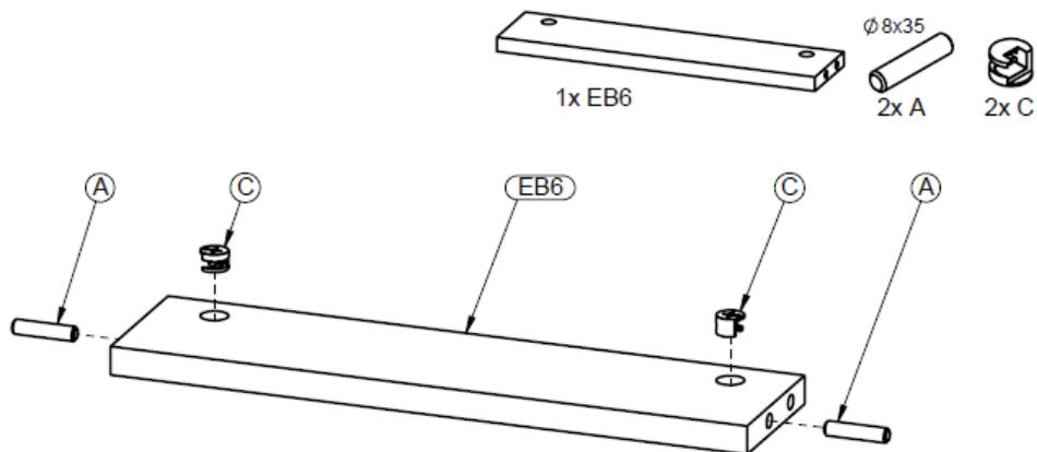
**Step 10 :** Use the the drawer back **EB6**, two wooden dowels **A** and two eccentrics **C**
