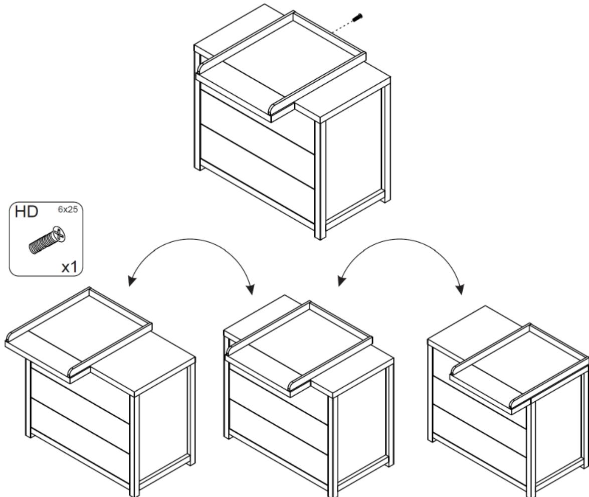
**Step 4 :** Use the parts of step 3, the Stripes chest of drawers and one bolt **HD**
