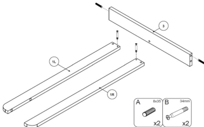
**Step 1 :** Use the sides **1L** and **1R**, the back **3**, two wooden dowels **A** and two connectors **B**
