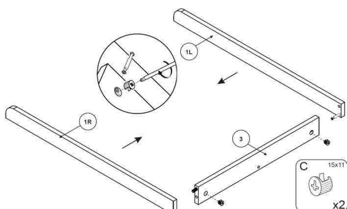
**Step 2 :** Use the parts of step 1 and two eccentrics **C**
